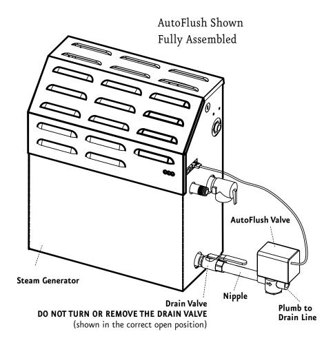
Our exclusive AutoFlush automatically and electronically drains the system, providing CleanSteam... Every Time and introduces fresh water.
