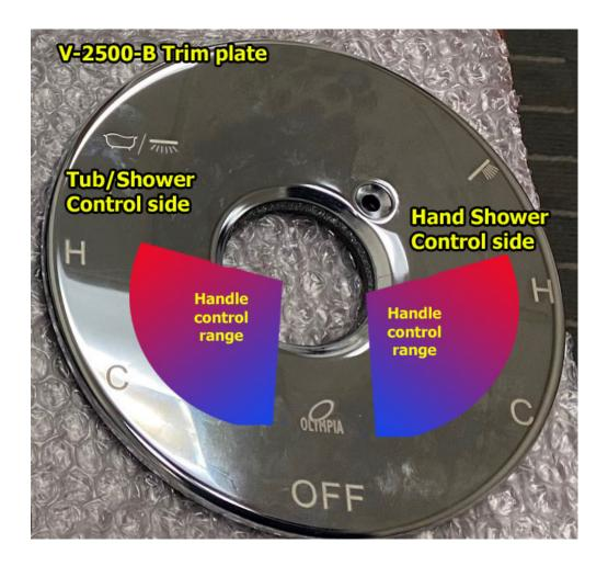
When the handle is in the six o'clock position, the valve is off. Counter-clockwise controls the hand shower and clockwise controls the tub/shower ports.
