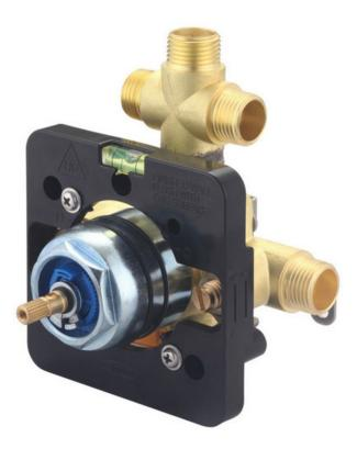
Prior to this valve, the method of piping in a hand-held shower was to run mixed<sup>1</sup> water off the pressure balance to a diverter valve. The user then had a choice to select the water to be routed to the shower head or the hand-held shower. This required a separate valve and trim and space on the wall.
